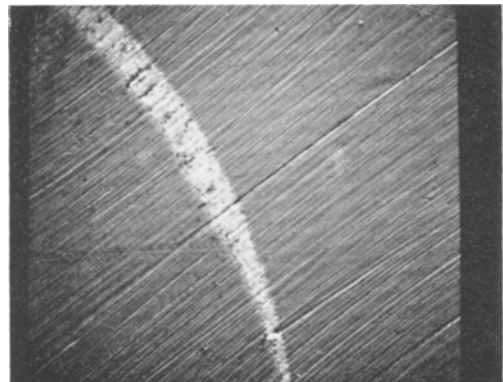
Figure 6 Illustration of atomic number contrast. A view of the soldered boundary between two concentric brass tubes. The soldered joint appears much brighter ( \times 47 ).
