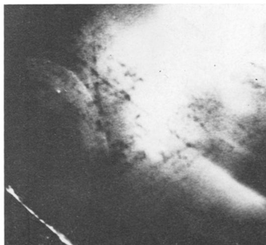
Figure 16 Image of GaAs in the cathodoluminescent mode. Visible are crystallographic defects ( \times 000 ). (By courtesy of R. Wayte.)
