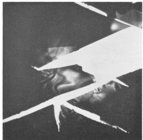
Figure 15 Bend contours in electro-polished austenitic stainless steel observed in the transmission mode ( \times 64 ) (By courtesy of Cambridge Scientific Instruments Limited).
